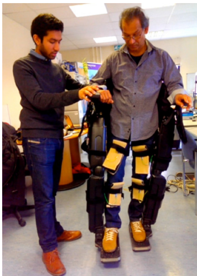
Fig. 1 Testing interaction force data acquisition at the pHRI
